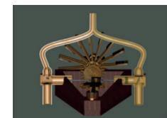
Figure 5: 3D-model recreated by FSTC of the reciprocating pump with a water wheel as the drive source. To see animation of the pump
